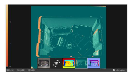
The color scale represents the variation in the SNR values. A pixel found at the higher end of the color scale represents a point associated with strong signal quality. For a point associated with a pixel found at the lower end of the color scale the ratio is more influenced by noise. Hence, these points involves higher uncertainty.
