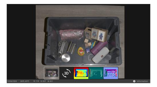
When doing a 2D+3D capture with different pixel sampling you can switch between the 2D image from the 2D capture and 3D capture in the top-left drop-down.
