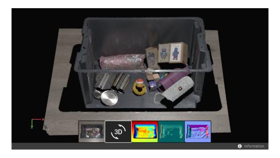
Turning color ( C , D and R ) and mesh ( M ) on and off in this view helps evaluate the point cloud quality. The point size is also adjustable through the drop-down menu at the top left. Adjusting the point size is for example helpful for inspecting areas where textures are important. If you have enabled the Region Of Interest, you can also modify the visibility of this in the drop-down menu.
